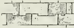
STONE CUTTING, FIG. 1: WITH JOGGLED JOINTS, GIVING GREAT SOLIDITY TO THE WORK; SYRIA, 4TH CENTURY.
